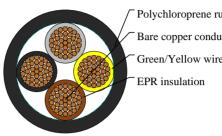
Polychloroprene rubber outer jacket Bare copper conductor Green/Yellow wire
